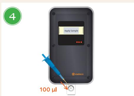
Apply contents of 100 µl pipette to the cartridge well. The reader will detect the sample within 60 seconds of application and will initiate an automatic 9-minute countdown.
