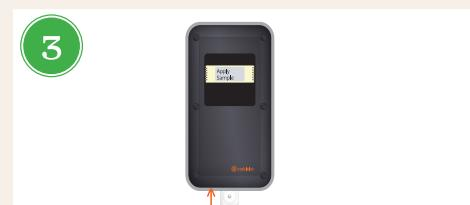
Ensure that the switch is positioned to the left for Standard mode. Insert a blank test cartridge into the reader. The reader will turn on automatically and display "Apply Sample".
