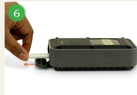
After the SAA result is displayed and recorded, remove the test cartridge and insert the next as each additional test reaches the 10-minute mark.\*\*
