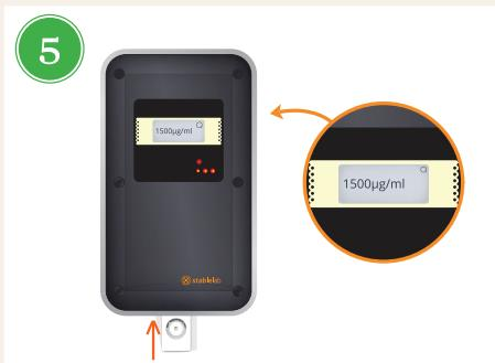
After 10 minutes, insert the test cartridge into the reader. The Test and Control window should be facing up and forward. The reader will power on and the result will be immediately displayed for 20 seconds before being permanently deleted from the device.
